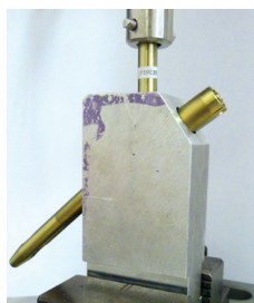
Set Screw Failure Test Set Up
